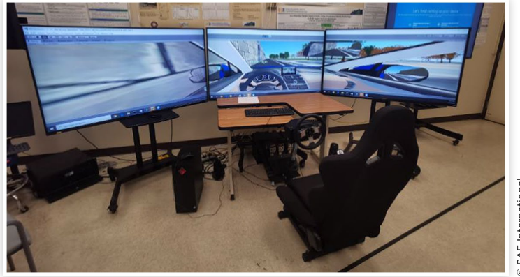
FIGURE 3 Hardware setup for HuiL in a lab environment.
