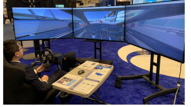
Fig. 4. Driving simulator platform built on Logitech Racing Wheel and Unity.
