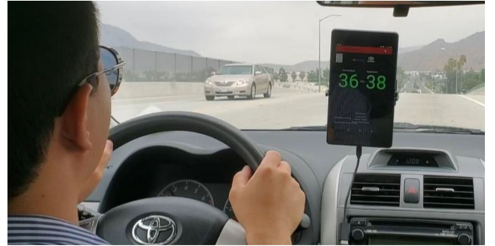
Fig. 8. A driver is tracking ASA on HMI in a real passenger vehicle.
