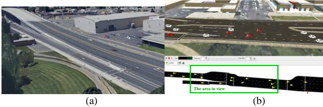
Figure 4. The Integrated Simulation based on a Real-world Ramp Merging Area in Riverside, CA: (a) View from Google Maps at the real-world ramp; (b) User interface of the Unity-SUMO co-simulation framework.
